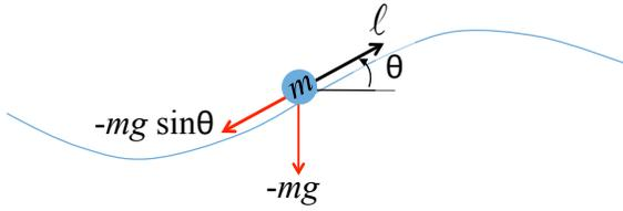
**Figure 1.3:** Definition diagram for the car-parking example.
